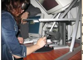
Besides, they also invent a set of virtual reality system using the skill of force feedback to stimulate moxibustion therapy. Through the equipment, users can stimulate moxibustion to decrease the dangers in a real situation. However, there is still a lot of room for the equipment to make progresses.
